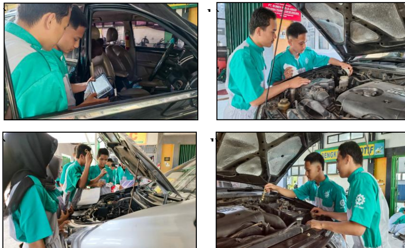
Figure 3. Car Inspection Process: a) Scanning Damage to the EFI System; b) Checking the Oil; c) Engine Oil Check; d) Re-examination
